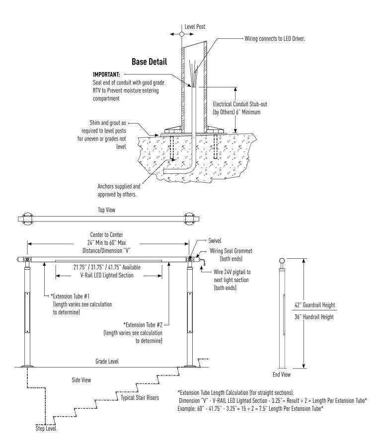
IVR2-SPI: 2" Slim Post Integral Power Supply (Post Mounted)
