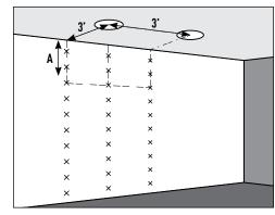
Example: Two luminaires located 3' from wall and spaced 3' on center, the illumination on the wall 3' down from ceiling will be 18fc beneath units and 22fc between units
