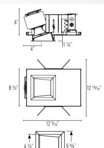
Ceiling Cut Out: 5 1/4" x 5 1/4" Maximum Ceiling Thickness: 1 1/4" Minimum Ceiling Thickness: 1/2"
